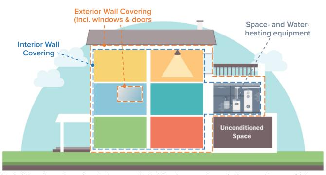
The **building thermal envelope** is the parts of a building (e.g., exterior walls, floors, ceilings, roofs) that enclose conditioned space or provide a boundary between conditioned and unconditioned space. **Conditioned space** is an area or room that is normally heated or cooled by equipment, whereas **unconditioned space** is any enclosed space within a building with no equipment to regulate temperature, like garages or attics.
